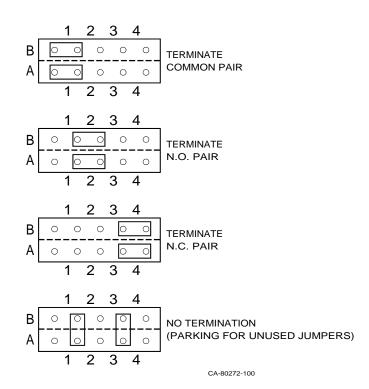
Figure 2. 600 Ohm Termination Jumpering E9-E16
